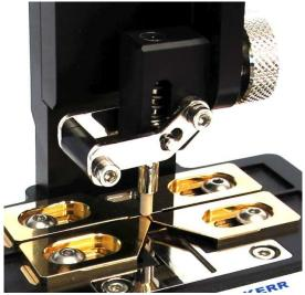
10324 showing 4-terminal connection DUT fits under vertical plunger
