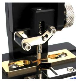
1032 showing 2-terminal connection DUT fits under vertical plunger
